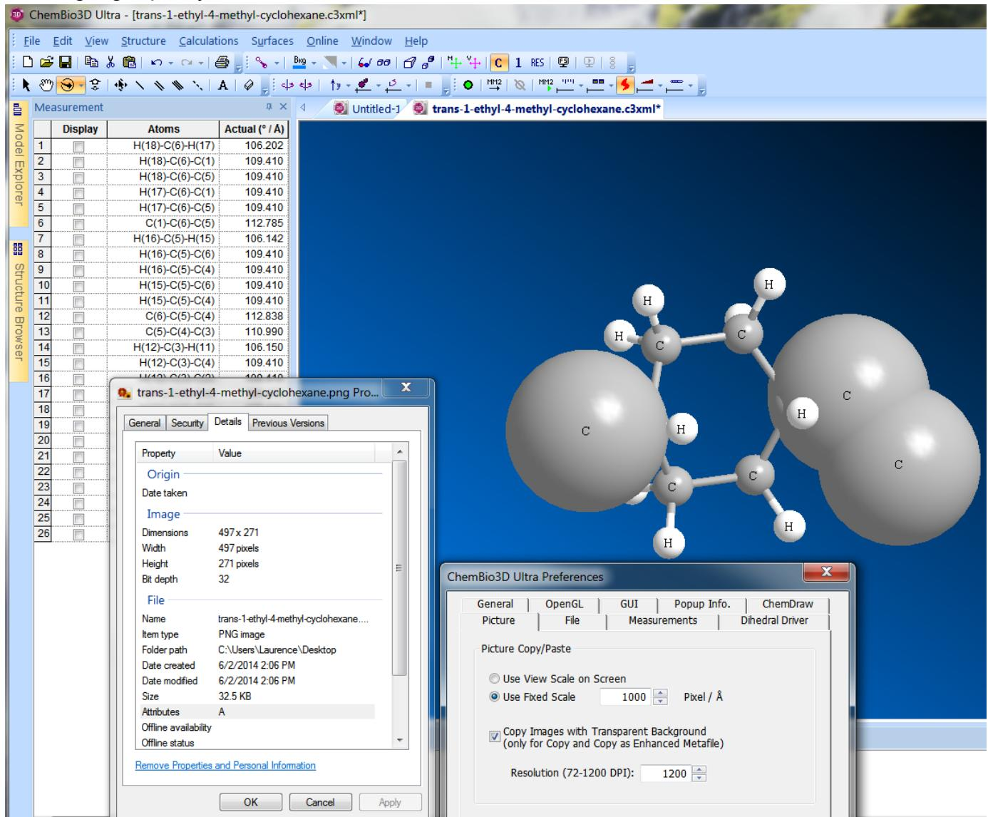
Using settings in ChemBio3D (right box) gives high resolution PNG file (32-bit depth).
